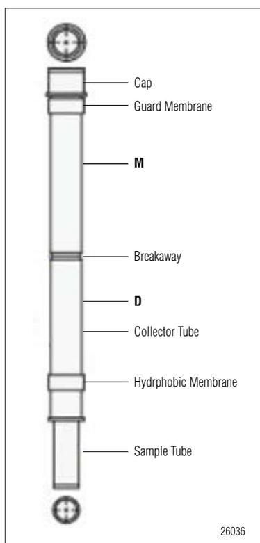
Figure 1. MICRO DIST tube assembly<sup>14</sup>
