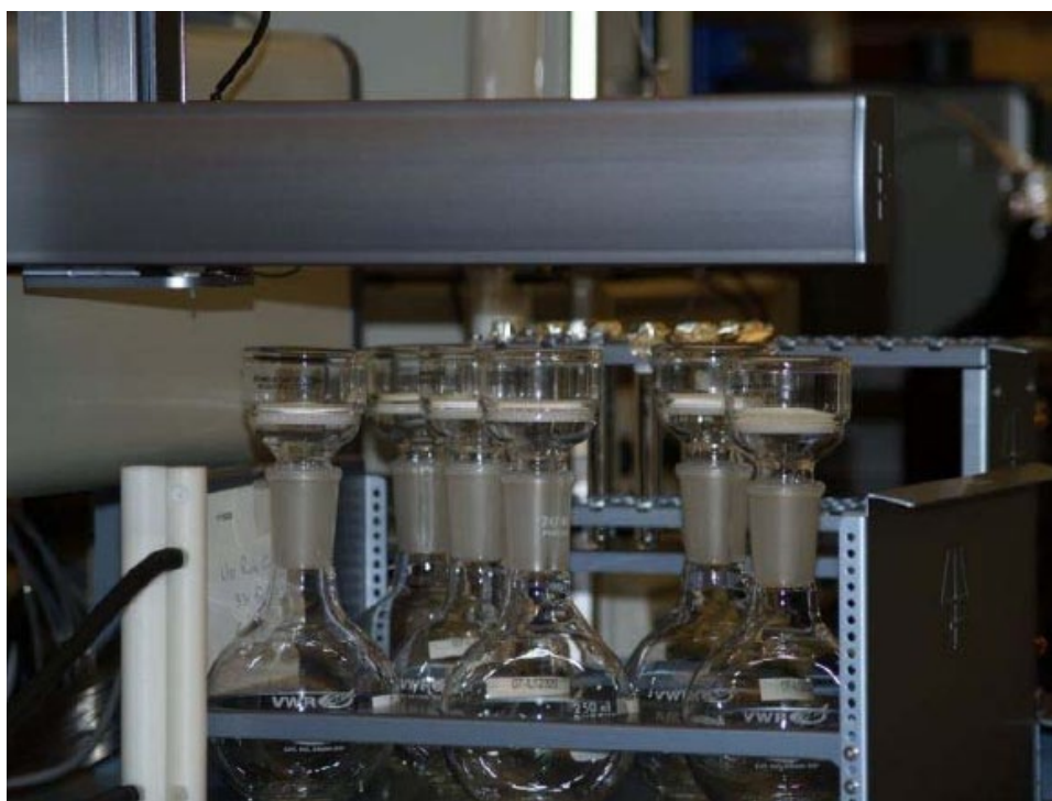
Figure 1. Using Evaporation Flasks With Fritted Filters on the Automated Gilson GX-271 GPC Clean-up System.
