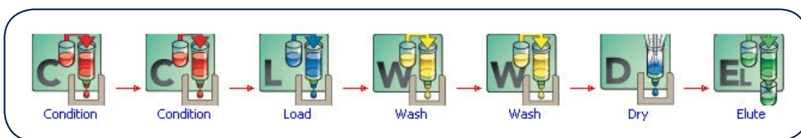
Figure 2. TRILUTION LH SPE Tasks for Extraction of Fipronil and Bifenthrin from Honey.
