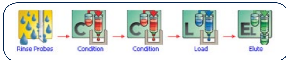
Figure 1. TRILUTION LH SPE Tasks for Extraction of Sweeteners from Water.
