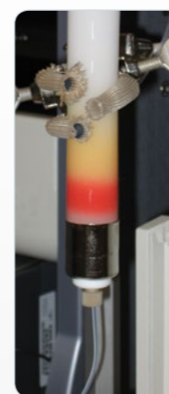
Example of separation of high and low molecular weighted analytes.
