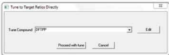
Figure 2: Tune-to-target for EPA tuning compounds are selectable in the software, and ratios can be easily edited if further optimization is required.
